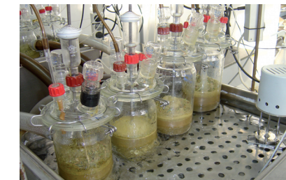
Simulation systems of ruminal fermentation
